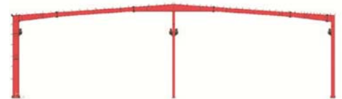
Nonprismatic sectional solid webbed frame.
