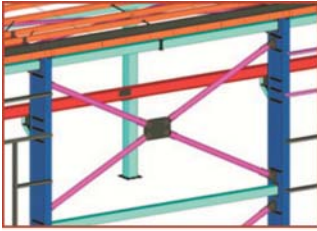
Central façade bracings.
